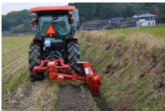
Open channel construction using a trench digger
